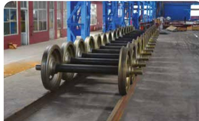
Our railway wheel production plant has capacity of 200.000 wheels in a year. Wheels for freight wagon, passenger car, high speed train, light rail system and locomotives with diameters from 700 mm to 1250 mm produce according to EN 13262+A2 standards.
